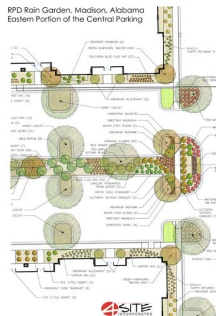
4Site illustration—eastern portion of central parking. Civil 3D and Storm and Sanitary Analysis helped to accurately model infiltration of rain water. Image courtesy of 4Site, Incorporated.
