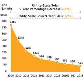
— Crystalline Utility-Scale Solar LCOE Mean
