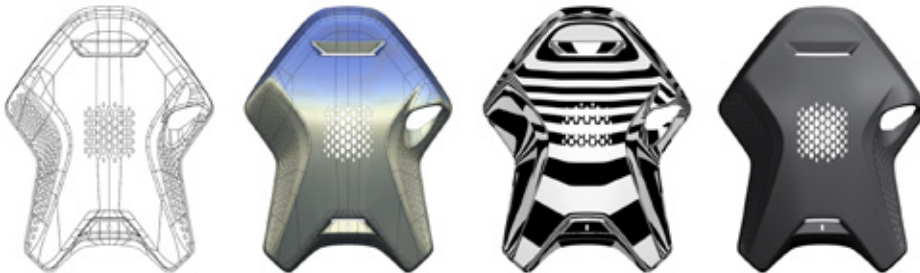
Autodesk ALIAS Surface translates product sketches to create customisable designs using fast concept modelling and high-quality precision surfacing functionalities
