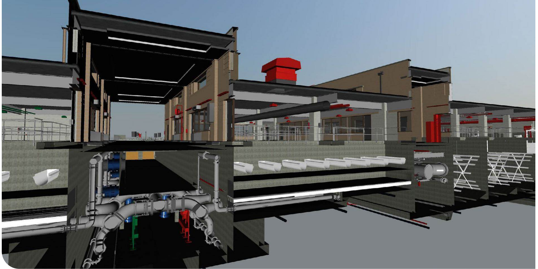
A 3D model of the Basin 7 main gallery shows a piping assembly connecting treatment trains. Courtesy of Arcadis.
