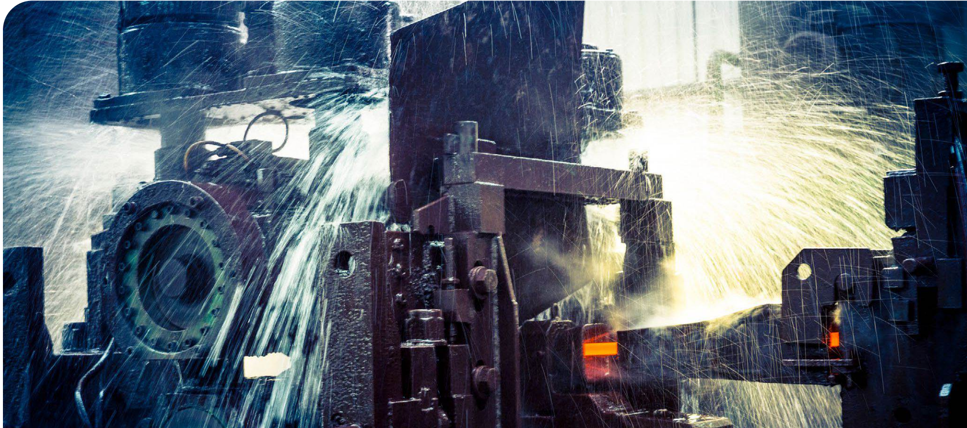
Water cools a rolling mill.
