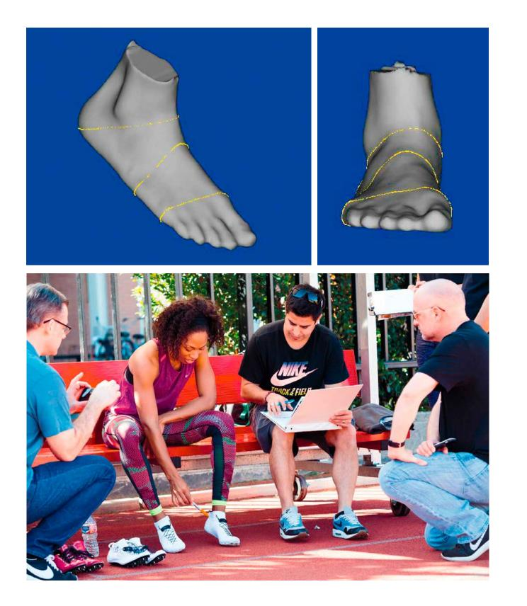
opposite top: Nike's 3D foot scanner captures 0.1 millimeter microslices of a runner's foot to build an accurate model. opposite **bottom:** Felix's subjective impressions to iterations of the shoe were important in evolving its design.
