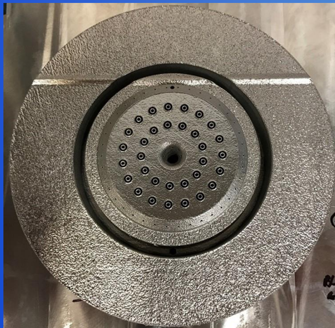
Injector test. Build time - $5.5k, Powder - $ 0.32k (5.82 kg), Saw - $0.2k, Plate resurface - $0.2k, Unsuccessful total - $6.22k. Successful total $6.22k. Total Cost $12.44k. 15 minute long simulation.
