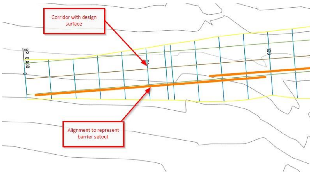
Figure 37: Corridor surface and Alignments
