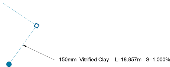
Pipe Labeled with 'Pipe Length and Slope'
