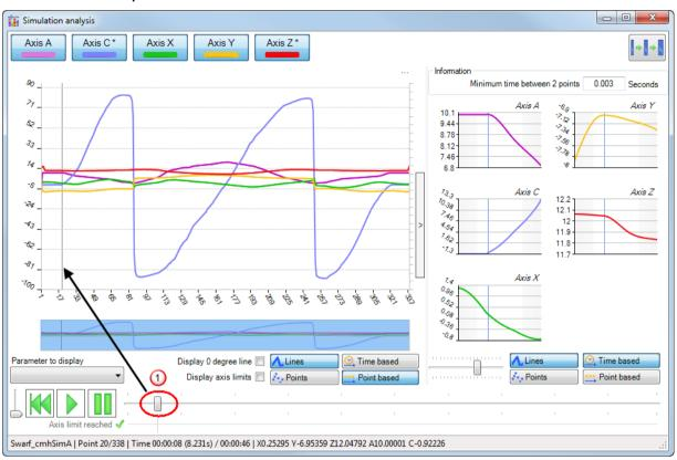
The individual graphs show the axis movement around the current simulation position (0).
