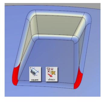
The key to success on all the corners is to align the CVs of the blend surface with the Hulls of the main fillet surfaces.
