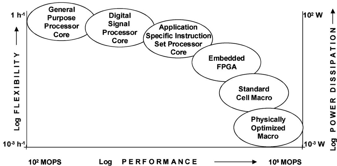
Figure 2.3: From[38], flexibility, power dissipation and performance of different digital design approaches. Flexibility is measured in the reciprocal of the design time.
