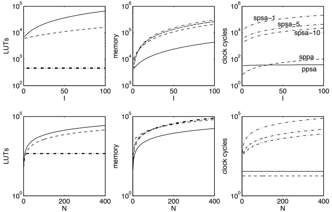
Figure 2.8: From [330], comparison of hardware resources and speed of different architectures (the SPSA architecture with 1, 5 and 10 PEs) with different number of inputs (I) and number of neurons (N).
