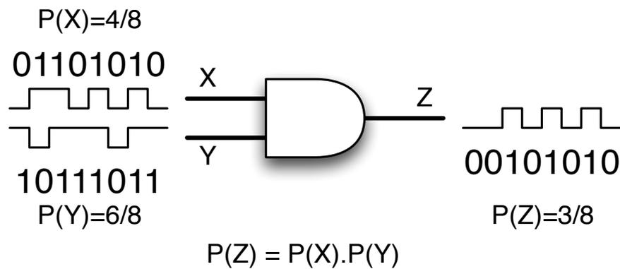
Figure 2.7: A simple example of computing product of two stochastic signals represented by 8-bit long random bitstreams using a single AND gate.
