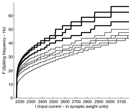
Figure 4.11: The effect of moving the middle control point (of figure 4.6(a)) on the F-I curve of the digital neuron. The bold lines are results of the middle point higher than zero.
