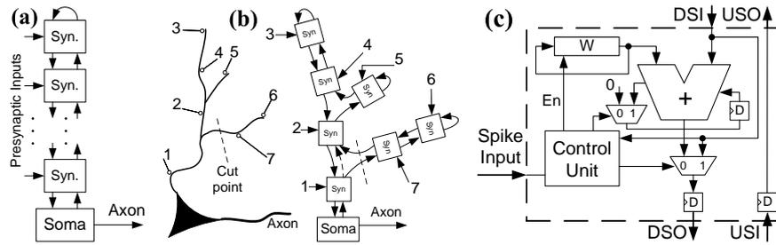
Figure 4.5: a) General architecture of the digital neuron (Syn=synapse) b) Example of the dendrite structure and its adaptability c) Synapse unit architecture.
