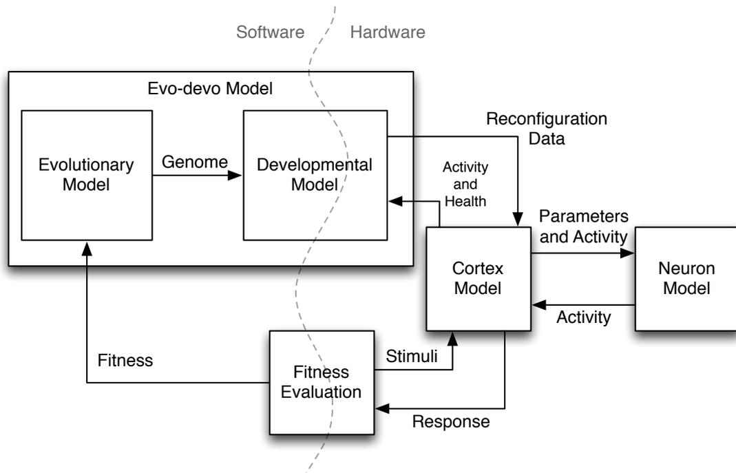
Figure 7.1: An abstract data flow diagram showing the interactions between different models in the system and demonstrating the hardware-software partitioning problem.
