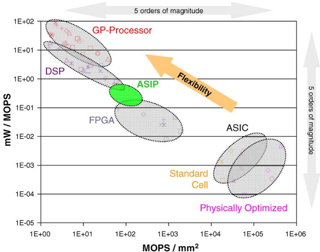
Figure 2.2: From [278], energy and area efficiency of different digital design approaches.
