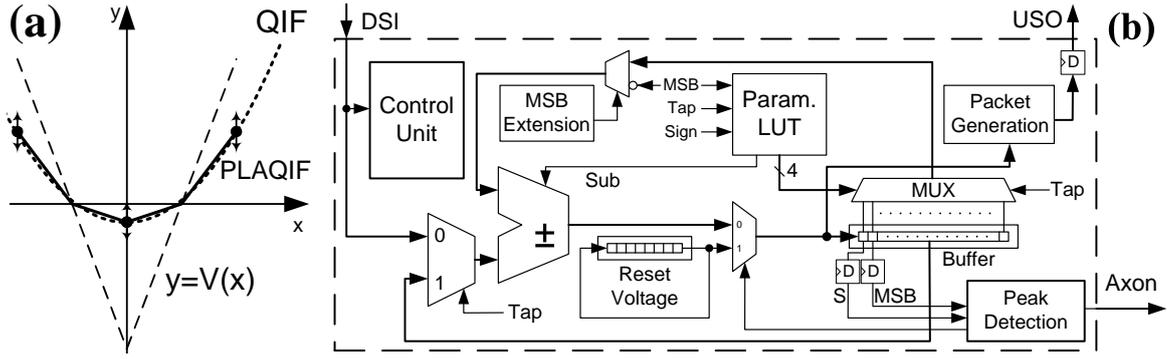
**Figure 4.6:** (a) The PLAQIF model approximates the QIF model (the dotted curve) with a piecewise linear function by modulating the V-shape function  $V(x)$ . The control points (arrows) can be moved by tuning the parameters. (b) Soma unit
