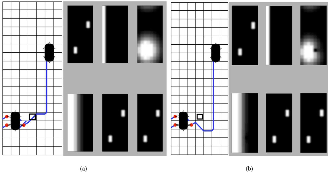
**Figure 6.17:** (a) The single axon routed from one neuron to the other along with the diffusion pattern of six proteins in the cortex. (b) The axon diverted to bypass the “faulty” glial cell (marked with a black square) along with the affected protein concentration pattern.
