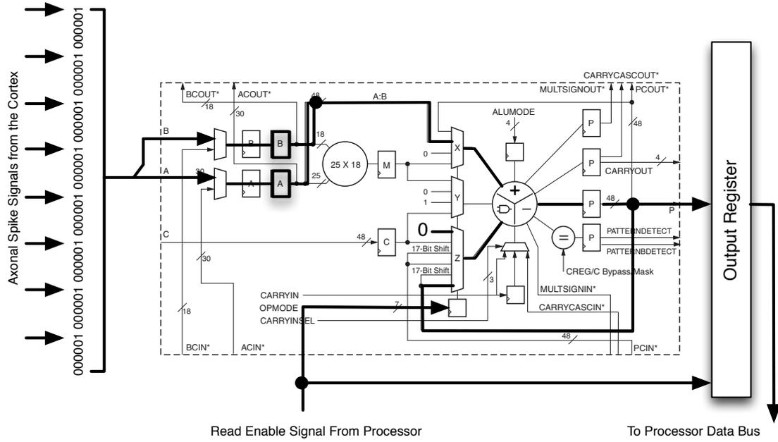
Figure D.1: Block diagram of the Spike Counter module with configuration of the DSP block as eight 6-bit counters.
