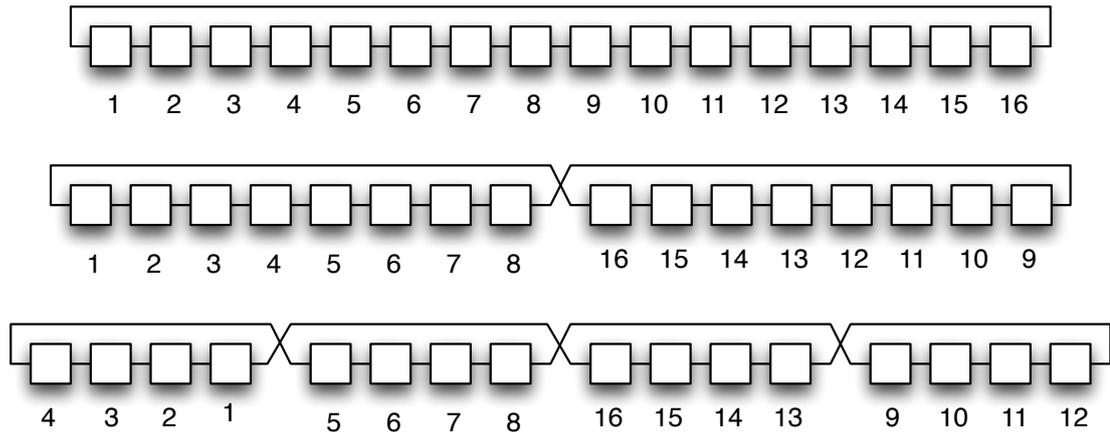
**Figure 5.16:** Solution to wrap-around wire delays in a 16 node ring network. The top connectivity pattern involves a very long wire between the first and last nodes while other links are very short. In the second pattern this delay is divided in half between two wires by flipping right half of the nodes. In the third pattern a quarter of the nodes at each end of the ring are also flipped again to cut the delays in half again.
