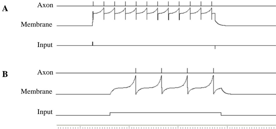
Figure 4.9: Traces of the input current, membrane potential, and the axon output of the digital neuron in the first experiment: **A)** Bistable behaviour ( $u_{reset} = 17000$ ). **B)** Monostable behaviour ( $u_{reset} = -16384$ ).
