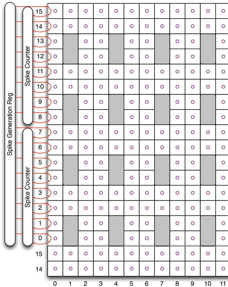
**Figure 5.8: Spike Counters and Spike Generators as IO cells connected to a sample 16x12 cortex. This figure also shows the spike signals being looped back in to the IO cell for verification and testing of the spike generator and counter modules.**
