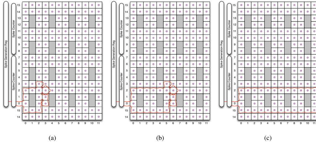
**Figure 5.9:** Three examples of test cases for testing axonal signal routing around soma cells on the cortex. The particular shape in (a) and (b) insures that every different switch state is at least once tested through an axonal path.
