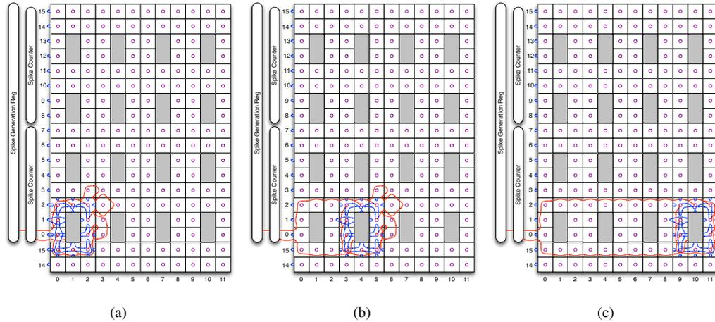
**Figure 5.10:** Three examples of test cases for testing dendrite signal routing around soma cells on the cortex. The particular shape of the dendrite in (a) and (b) tests all possible different switch states through a single dendrite loop.
