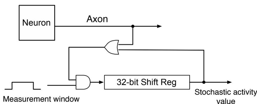
Figure 5.3: An example of a circuit that can be used to gather stochastic measurements of the activity of a neuron over a measurement period.
