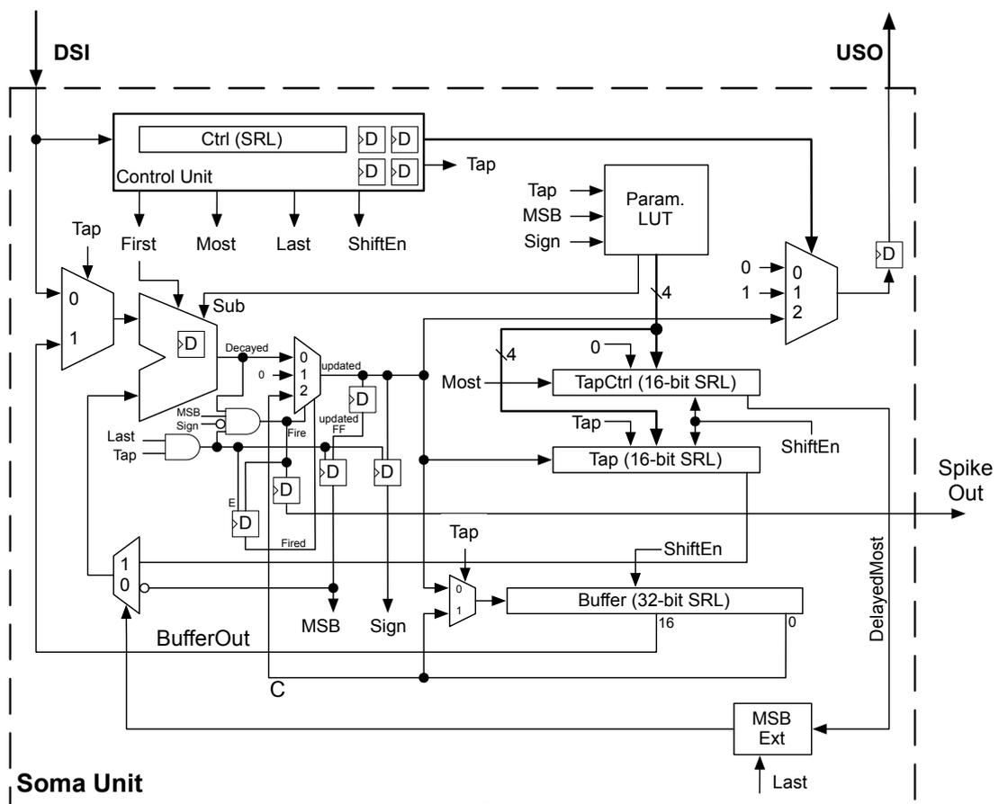
Figure 4.7: Detailed block diagram of the soma unit design.
