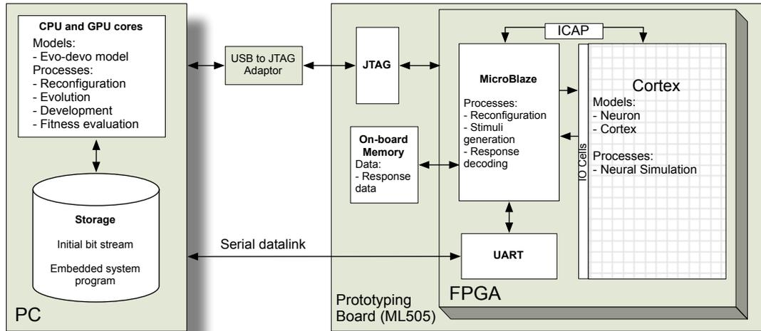
Figure 7.5: A block diagram of the integrated system of the case study showing the connectivity of the main components (PC and FPGA) and mapping of the modules and processes to these components.
