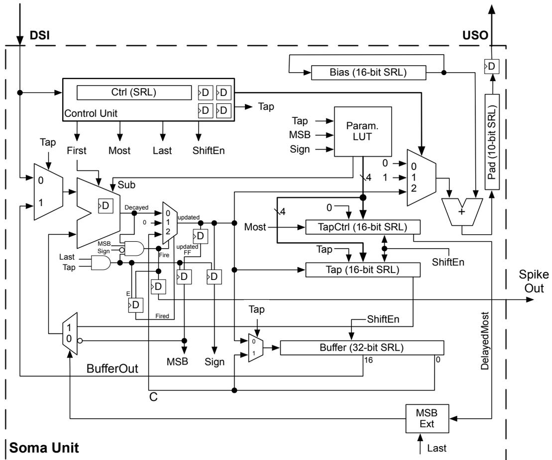
Figure 5.14: A detailed diagram of the revised soma unit showing the bias register, serial adder and padding shift register that were added to the soma unit. The global reset and clock signals are not shown here.
