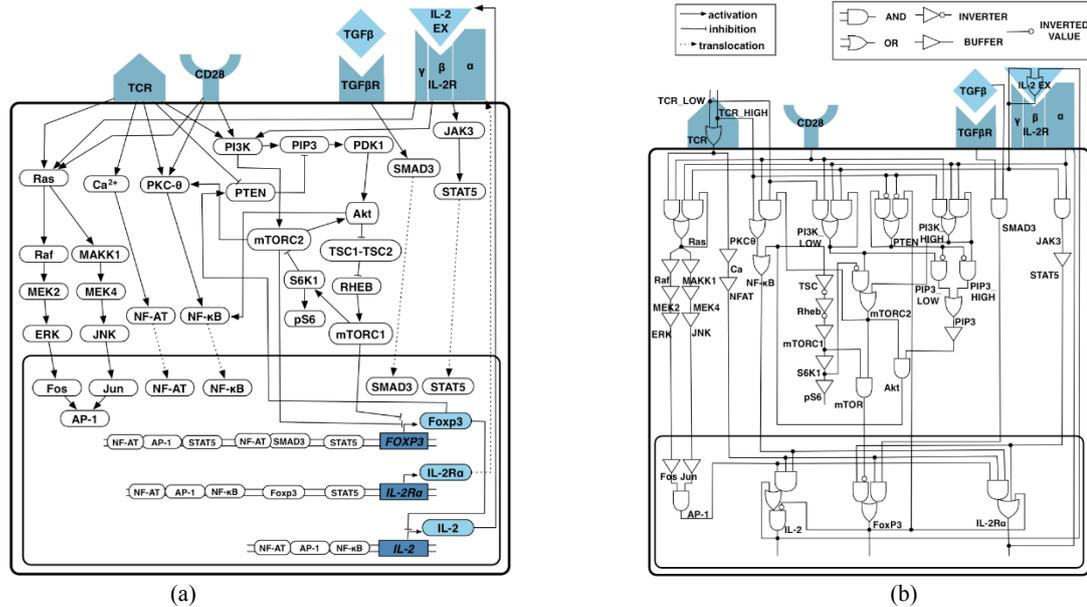
Figure 6.6: Example of translating a biological GRN into a stochastic asynchronous logic circuit (T-cell differentiation network from [267]). a) Molecular interaction map of T-cell differentiation GRN. b) Gate-based logic implementation of the same GRN.
