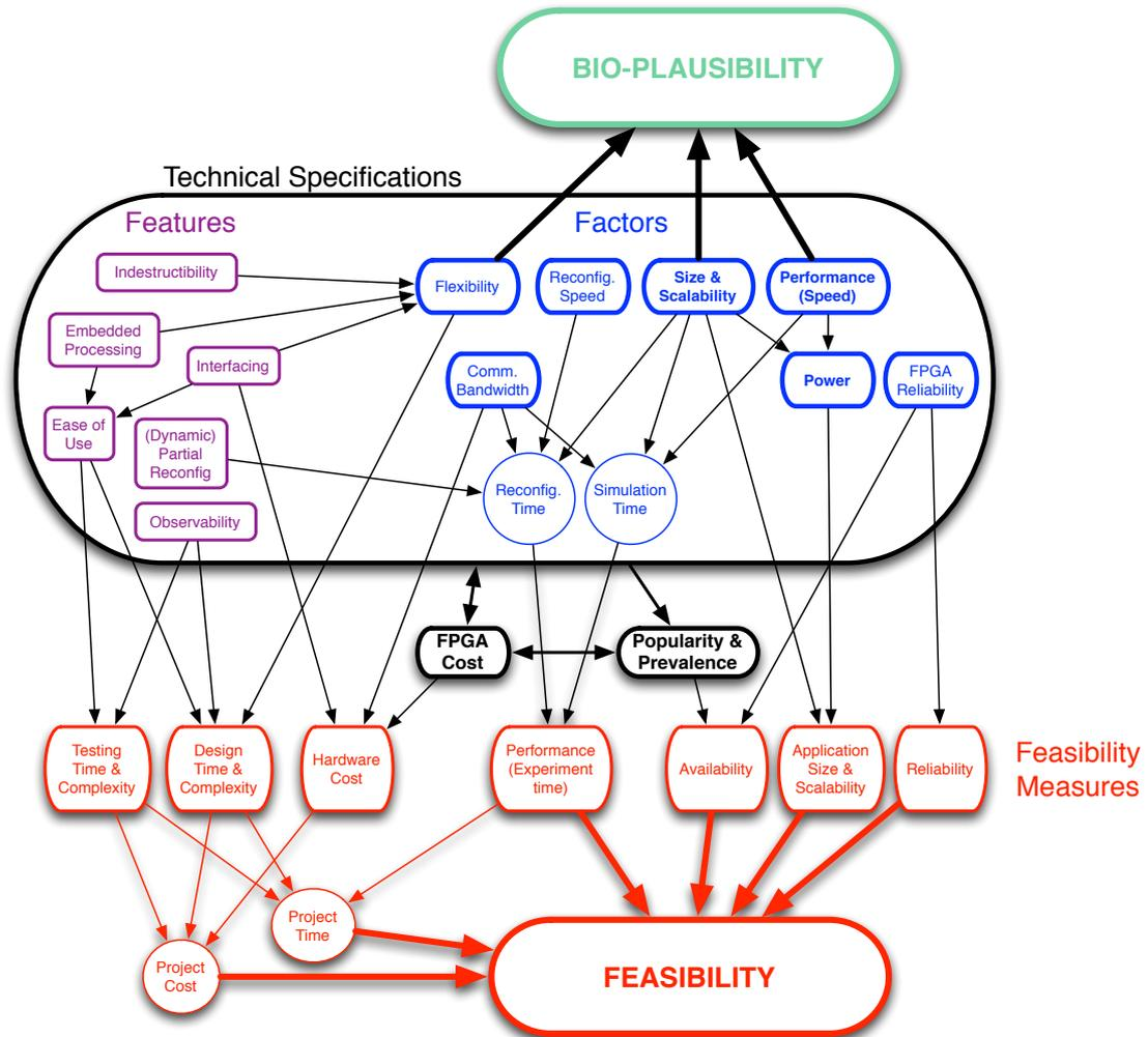
Figure 3.2: Detailed trade-offs and interactions between different technical features and factors involved in the selection of the FPGA platform and how they affect the feasibility and bio-plausibility of the whole system.
