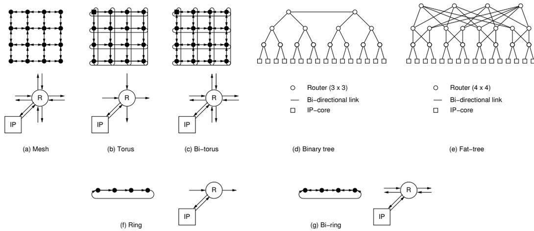
**Figure 5.1: Common NOC topologies along with their router(R) and PE (IP) connections and ports (From [328]).**
