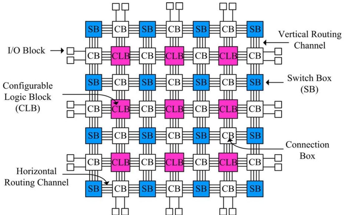
Figure 2.4: General conceptual of FPGA architecture [30]
