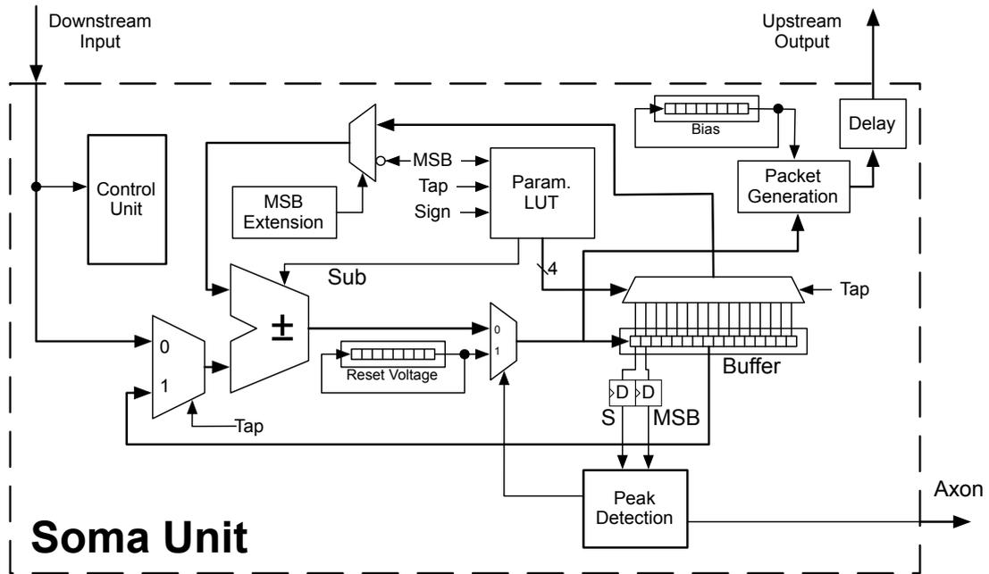
Figure 5.12: Block diagram of the revised soma unit showing the bias register, and the delay block that were added to the soma unit. The global reset and clock signals are not shown here.
