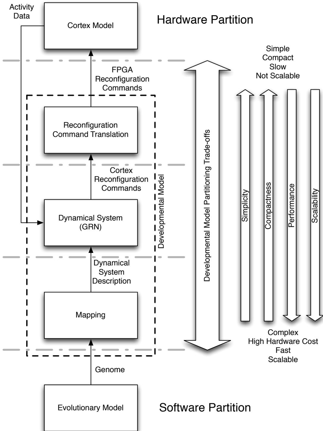
Figure 7.3: Developmental model partitioning trade-offs depicting the growth of different factors based on the partitioning boundary between hardware and software components of the system. The stroke dash lines represent some of the different options for the partitioning of the developmental model between hardware and software components.
