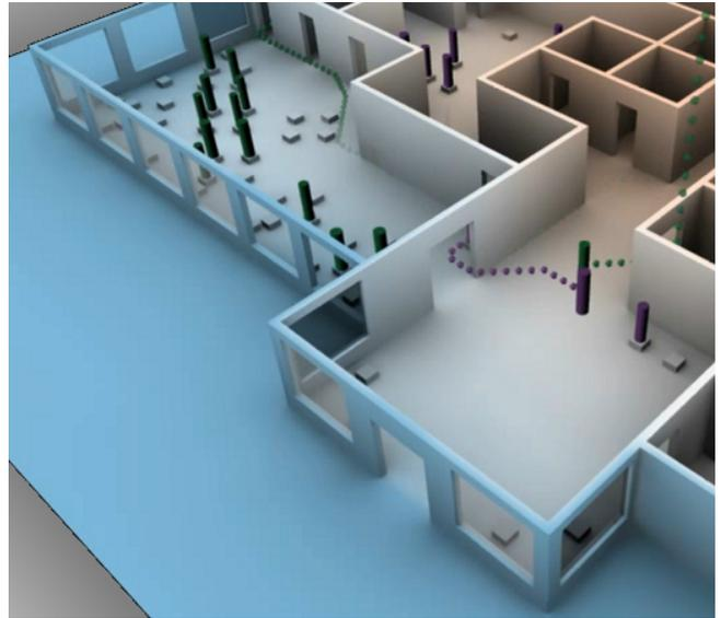
**Figure 6.** A virtual hotel modeled and simulated using DesignDEVS. The indoor temperature distribution (surface coloring) influences the window-opening behavior of occupants (cylinders), which in turn affects indoor temperature.
