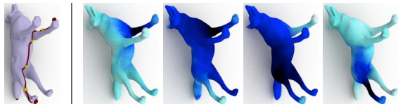
Figure 9: A soft map (right) between a straight and a bent wolf model constructed by optimizing \mathcal{E}(\mu) after fixing three points marked in red (left). The resulting distributions, constructed solely using continuity and constraints, are wide but have peaks aligned with their counterparts on the source.
