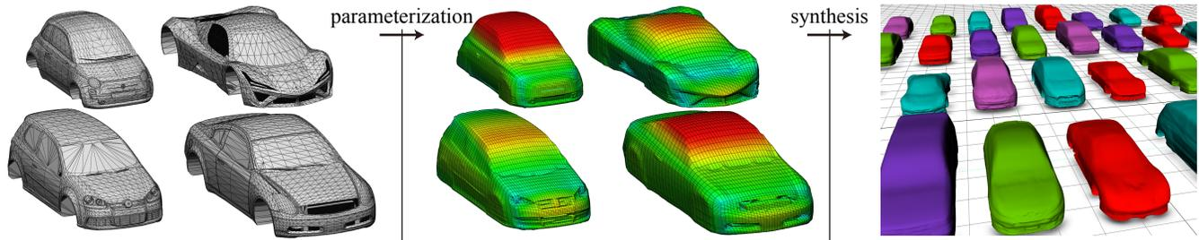
**Figure 1:** From unstructured triangle mesh (left), our approach can efficiently and robustly construct a quad mesh with a consistent topology (middle) that is compactly parameterized as a height map (shown in color contour). The autoencoder constructs a low-dimensional representation of the set of shapes to synthesize new shapes (right). Our interface allows the user to interactively guide the synthesis by directly manipulating on the shapes.
