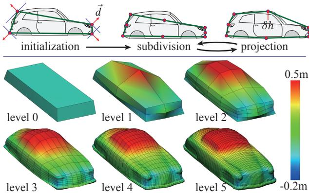
**Figure 2: Shrink wrapping parameterization. (top) 2D schematic illustration. (bottom) Example of parameterization in different subdivision levels.**
