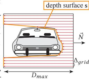
**2.1.1 relaxation.** The general non-manifold triangle meshes often have many holes (e.g., the gap between the doors, the air intake of the front grill). If a ray goes through such holes, it appears as a
