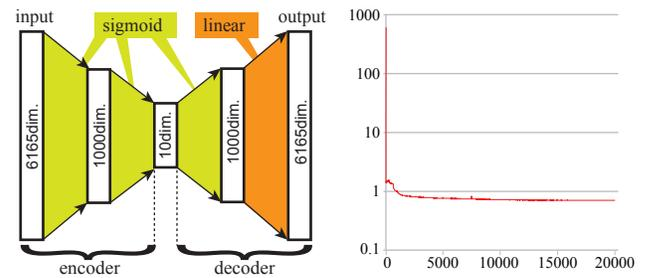
**Figure 3: (left) Configuration of our autoencoder network. (right) Convergence of the sum of squares in the training.**
