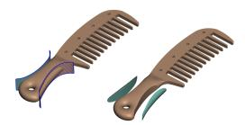
**Figure 7:** Creating a complex by cutting a model with sheets. Left: input comb and open surfaces. Right: result of thickening the open surfaces into volumes, performing a non-regularized Boolean operation, and discarding the exterior of the thickened surface (exploded view).
