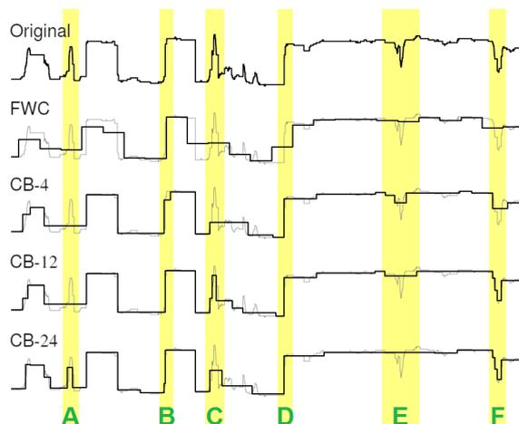
Figure 5: Light sensor data compressed with a 1-minute target resolution using different schemes
