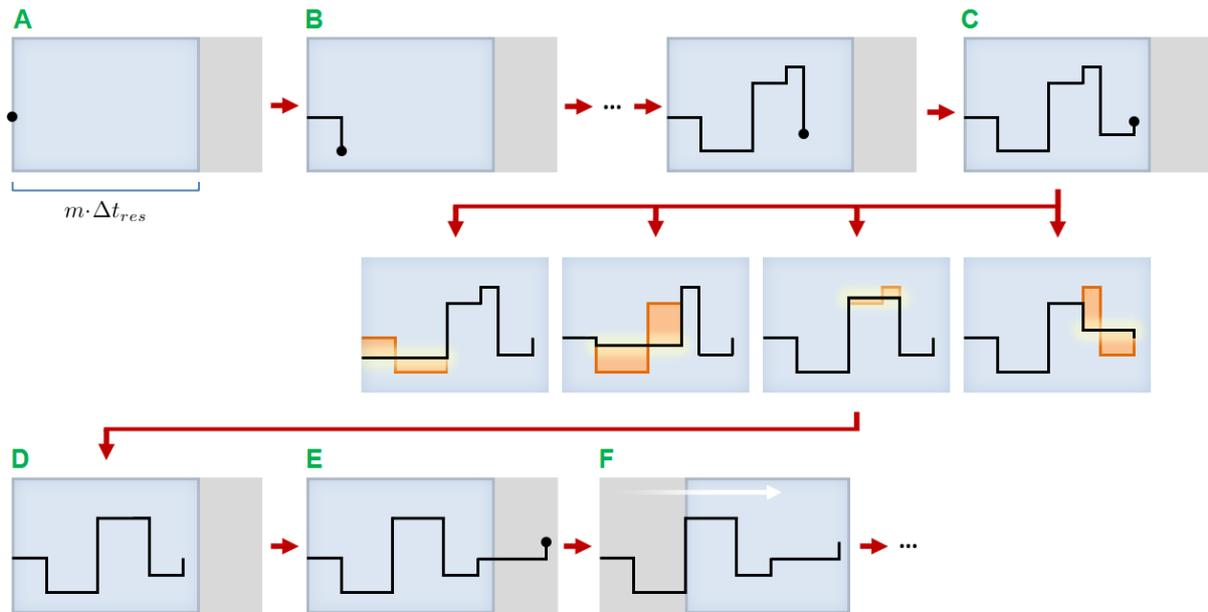
Figure 3: Example of real time compression. Segments shown on a blue background are in the compression buffer. Transition A – B shows the arrival of a datapoints within the buffer’s time window, C – D illustrates the selective merging of segments in a full buffer, and E – F shows the arrival of a datapoint beyond the end of the time window.
