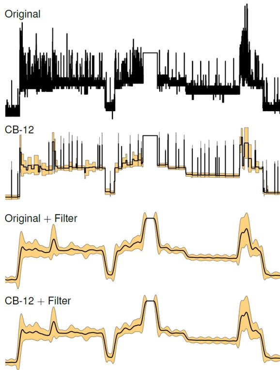
Figure 9: Electrical data with low-pass filtering applied to the original and compressed time series
