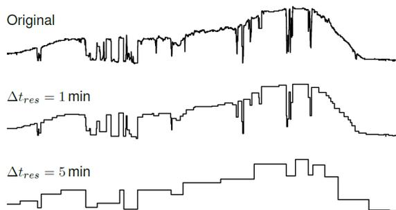
Figure 4: Light sensor data compressed with a size-12 buffer at 1- and 5-minute target resolutions
