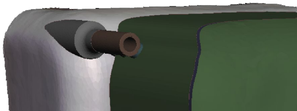
Figure 4: The mounting brackets allow the enclosure to easily be added to or removed from a legacy object.
