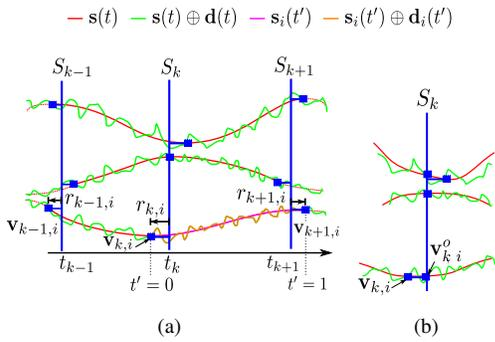
**Figure 3:** a) The staggered pose representation models transitions as a composition of splines (red) and displacement maps (green) to provide low-frequency editing controls that preserve detail. b) To facilitate direct geometric editing of poses, we include an additional knot at the pose time; this knot and the knot at the extreme value are mutually constrained to maintain continuity.
