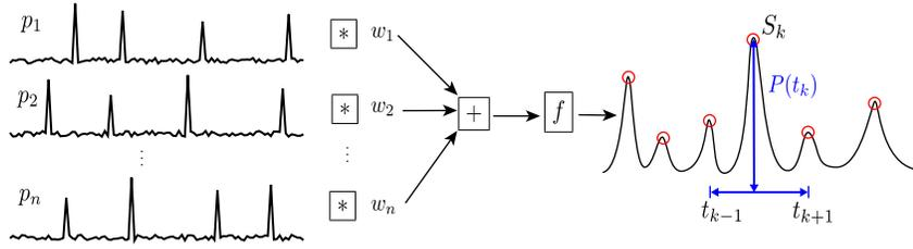
**Figure 5:** To locate staggered pose times, we combine signals that measure motion features, filter the result to combine close peaks into an overall probability, and select times at the peaks of this signal, prioritizing by probability and temporal locality.
