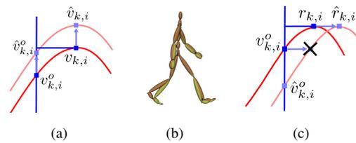
**Figure 6:** We mutually constrain editing knots and extreme value knots to maintain continuity. Change in value is copied from one to the other (a). The non-staggered pose, shown in orange, appears exaggerated relative to the true pose at the staggered pose time (yellow). Change in timing refinement requires spline evaluation and re-creation of the editing knot to maintain continuity (c).
