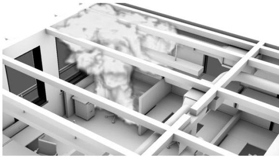
Figure 8: A volumetric rendering of hot buoyant plume.
