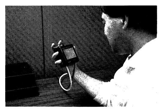
Fig. 8c. Third experiment condition consisting of a small 4-inch monitor, dynamic display using the palmtop virtual-reality system for input.
