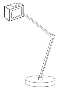
Fig 9 A holster for the palmtop to reduce muscle fatigue during prolonged use of the device
