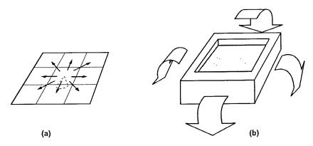
Fig. 2. Localized viewing of adjacent cells (a) can be achieved by making use of a tilting mechanism. The user pretends that the hand unit is resting on a pin. Tilting the unit (b) will allow for the appropriate adjacent cell to be viewed.
