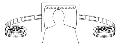
Fig 12. Film reel metaphor in which data placed on the surface of the film can be viewed in detail by the conventional computer monitor. The palmtop unit serves as a means for advancing or rewinding the film and to preview portions of the film not currently shown on the main monitor.
