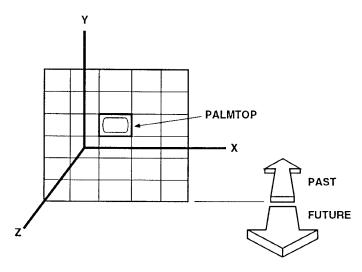
Fig. 1. Virtual cubic spreadsheet. The hand unit displays one cell of the spreadsheet at any given time. As a user moves the unit to different spatial locations, the appropriate cell of the spreadsheet is shown in the display of the hand unit. In this instance the z axis has been associated with time; past events are further away, and future events are closer to the person holding the palmtop.
