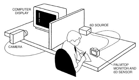
Fig. 4. Configuration of the Chameleon prototype.
