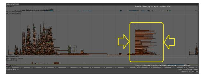
Here the Profiler shows many separate identical tasks that start at nearly the same time on different threads, each finishing at different times. This type of profile offers a clue that there might be some shared resource that many threads need to access simultaneously.
