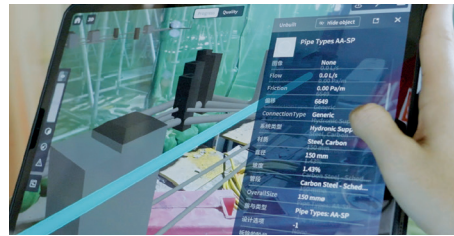
Virtual three-dimension models with physical reality for avoiding underground utilities damage Image Courtesy of Airport Authority Hong Kong and China State Construction Engineering (Hong Kong) Limited
