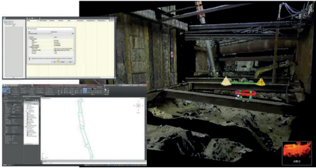
BIM and point cloud data integration for 5D earthwork calculation Image Courtesy of Airport Authority Hong Kong and China State Construction Engineering (Hong Kong) Limited
