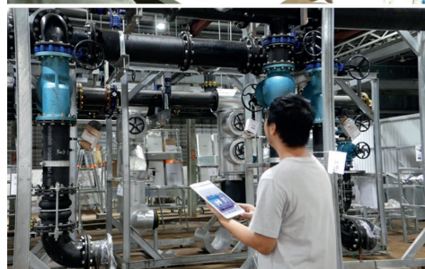
Standardization and DfMA of MEP modules enhances buildability, reduces time, cost and labour. Image Courtesy of ArchSD
