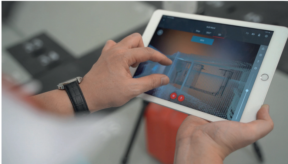
Point-cloud model generated by laser scan process Image Courtesy of Bureau of Public Works of Shenzhen Municipality and Architectural Services Department HKSAR Government and China State Construction Engineering (Hong Kong) Limited
