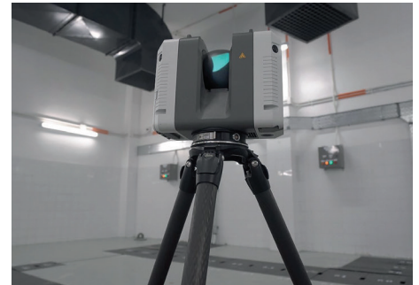
Laser scan process in the construction stage Image Courtesy of Bureau of Public Works of Shenzhen Municipality and Architectural Services Department, HKSAR Government and China State Construction Engineering (Hong Kong) Limited
