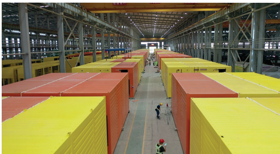
MiC production factory in China Zhuhai Image Courtesy of Bureau of Public Works of Shenzhen Municipality and Architectural Services Department, HKSAR Government and China State Construction Engineering (Hong Kong) Limited
