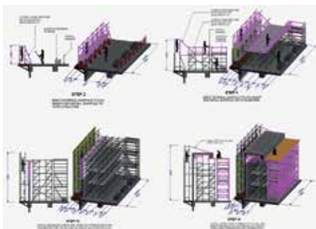
3D modeling helped scaffolding/ temporary works design and submission. Image Courtesy of Gammon Construction Limited and Hong Kong Science and Technology Parks Corporation
