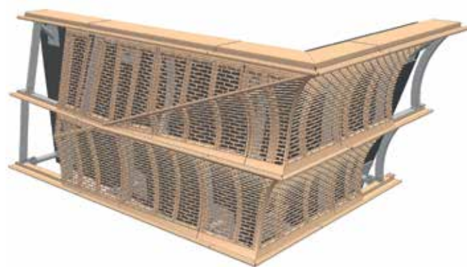
Digital Fabrication Model for External Perforated Aluminium Panel Image Courtesy of China State Construction Engineering (Hong Kong) Limited
