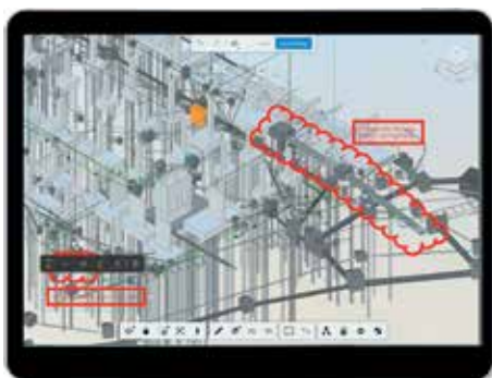
Instant comments on shop drawings and CSD submissions are done on BIM 360 Image Courtesy of ArchSD
