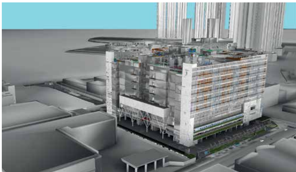
Coordination with a comprehensive BIM model including regional geography data. Image Courtesy of Gammon Construction Limited and Hong Kong Science and Technology Parks Corporation
