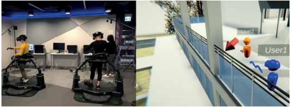
Two participants are performing design coordination tasks by using the MUVR motion simulator system in the physical world (left) and virtual world (right). Image Courtesy of City University of Hong Kong
