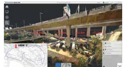
3D Scanning for Site Surveying Image Courtesy of Hip Hing Engineering Company Limited and Architectural Services Department, HKSAR Government and Vircon Limited
