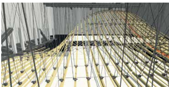
Construction Method Simulation for feature Ceiling Image Courtesy of China State Construction Engineering (Hong Kong) Limited
