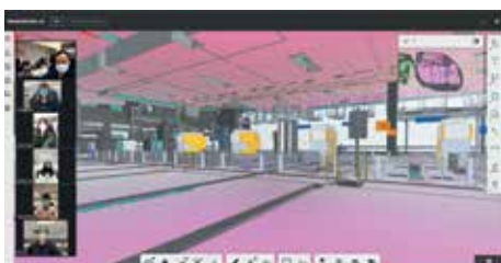
BIM Coordination-digital video conferencing software Image Courtesy of Hip Hing Engineering Company Limited and Architectural Services Department, HKSAR Government and Vircon Limited
