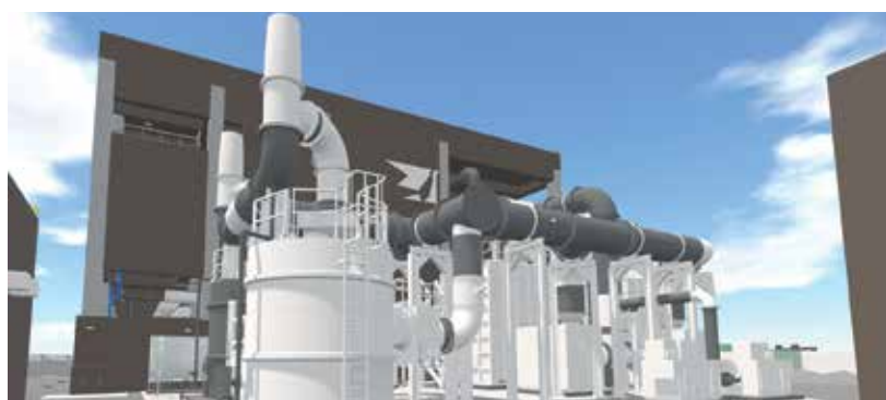
E&M Design of Deodorization Unit Image Courtesy of Drainage Services Department, HKSAR Government and AECOM Asia Company Limited and The Jardine Engineering Corporation, Limited
