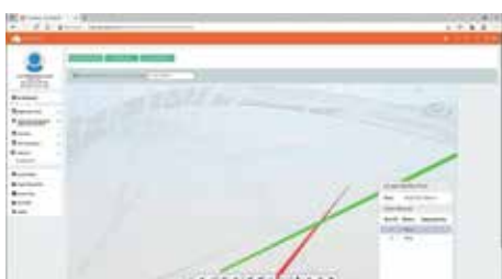
Automatic Clash Detection between Rock Bolts Image Courtesy of Drainage Services Department, HKSAR Government and AECOM Asia Company Limited and China State Construction Engineering (Hong Kong) Limited and MTECH Engineering Company Limited
