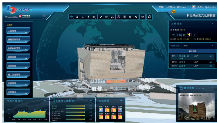
Smart Construction Platform for Hong Kong Palace Museum Image Courtesy of China State Construction Engineering (Hong Kong) Limited
