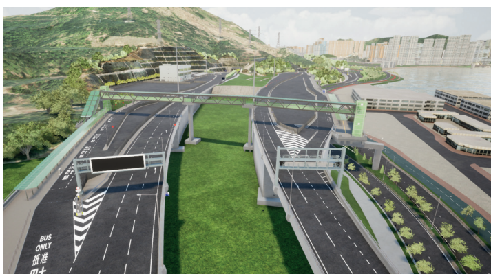
Design review in BIM model for lane control system (LCS) and road marking arrangement Image Courtesy of Gammon Construction Limited
