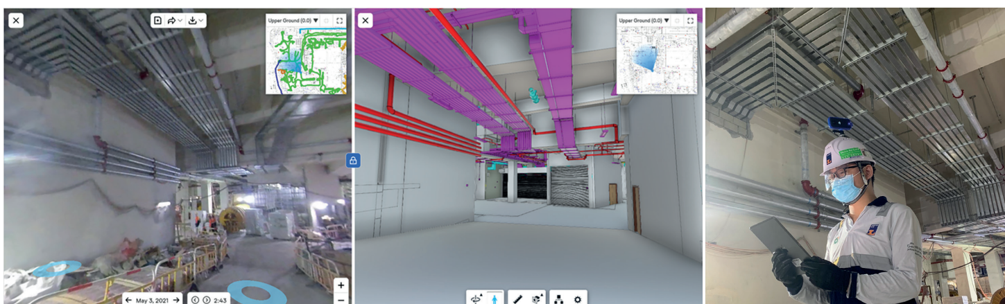
Daily project reality capture via 360 camera allowing for model comparison to existing work Image Courtesy of Leighton Contractors (Asia) Limited
