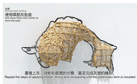
4D Animation illustrates construction sequence of plaster moulding Image Courtesy of ArchSD
