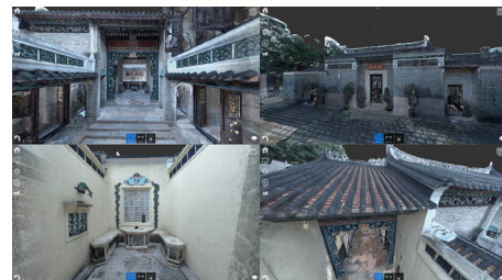
Generate 3D scan model from data collected on site Image Courtesy of ArchSD
