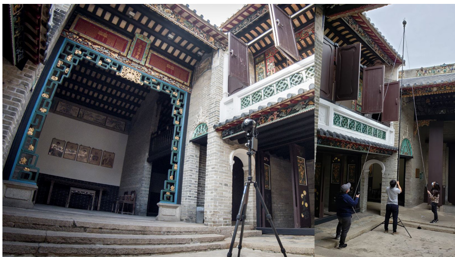
InstaPro 360 Degree Camera & Tripod for conducting 3D scanning works Image Courtesy of ArchSD
