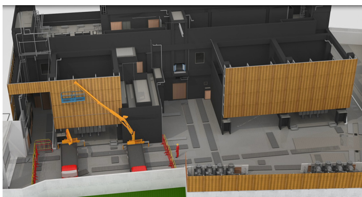
Construction Simulation of Metal Grille in Transformer Bay Image Courtesy of CLP Power Hong Kong Limited
