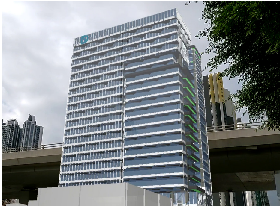
Visualize the entire building in AR (Hololens 2) and review the outlook on surrounding environment. Image Courtesy of Architectural Services Department, HKSAR and Shui On Joint Venture
