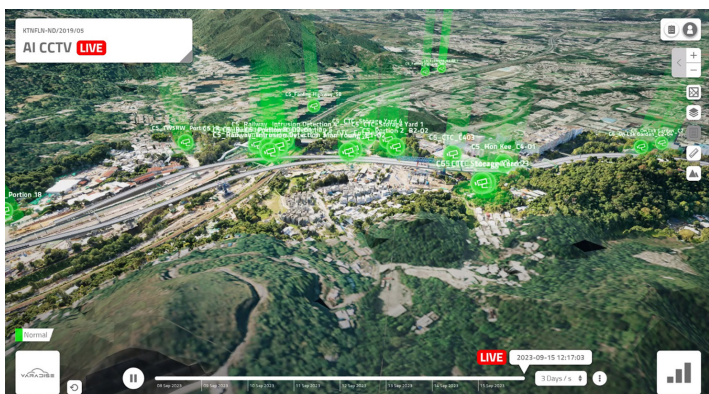
Centralised Management Platform (CMP) for Site Management and Monitoring Image Courtesy of Civil Engineering and Development Department, HKSAR Government and AECOM Asia Company Limited and CRCC - Paul Y. Joint Venture and Tyfron Consultancy Limited
