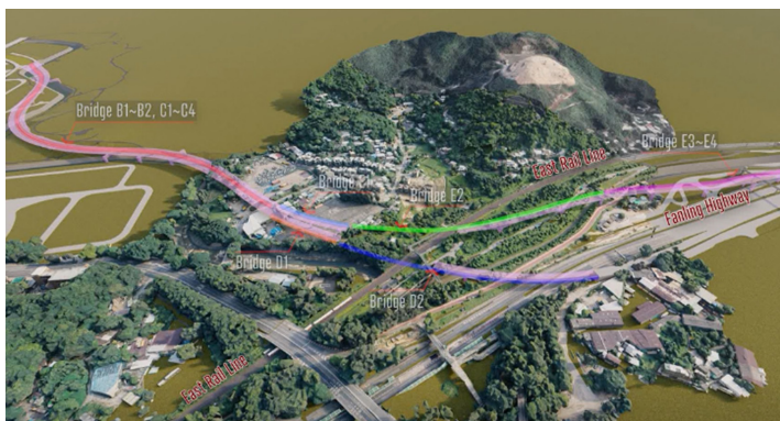
Integration of 3D survey and photogrammetry data for design and methodology studies Image Courtesy of Civil Engineering and Development Department, HKSAR Government and AECOM Asia Company Limited and CRCC - Paul Y. Joint Venture and Tyfron Consultancy Limited
