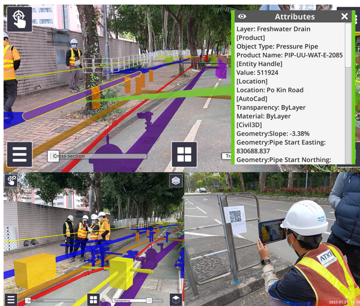
Visualization of Existing UUs or Planned Alignments by AR Technology Image Courtesy of WSD and Atkins and CWE and TYFRON
