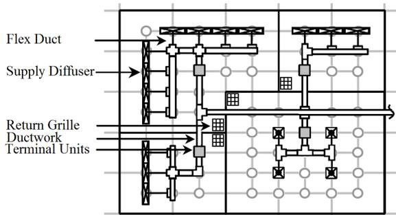
Figure 7. Example mapping of the HVAC system components.
