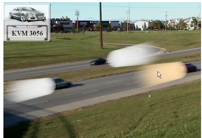
Figure 1 – Moving objects can be enhanced with a Comet to enlarge their activation area. We show its value in the case of a video feed (vehicle paths were annotated manually). When a car is selected more information (top left corner) is available.
