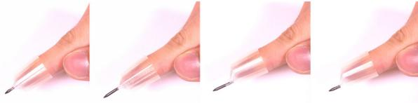
**Figure 2. A series of design variations were 3D printed to gain initial insights on the possible form factors. Shown above are two of the variations in nib position and nib length.**
