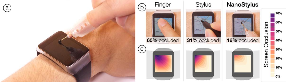
**Figure 1. a) The NanoStylus is a finger-mounted stylus which improves touch precision on ultra-small devices. b) Compared to direct touch and a traditional stylus, the NanoStylus significantly reduces occlusion. c) The heat maps show the estimated percentage of the display that is occluded when pointing at each coordinate on the smartwatch surface.**
