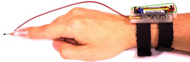
**Figure 3. The NanoStylus consists of a disassembled active capacitive stylus, housed in a custom 3D printed case that fits on the index finger. A circuit board and power source are mounted on an arm band.**
