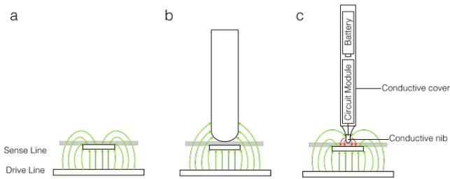
**Figure 4. a) Schematic of a capacitive touch screen. b) A passive stylus requires a large tip to trigger a touch event. c) An active stylus can achieve a smaller tip size by actively sending a negative charge to the sense lines.**
