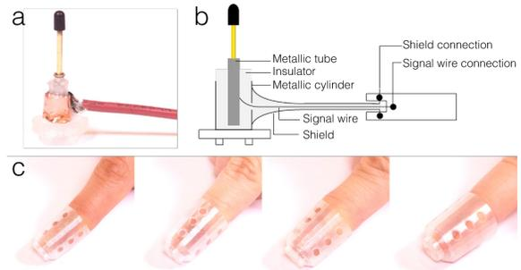
**Figure 6. a) The head was designed to hold the stylus nib. b) Connection between the head and the circuit board c) A series of case sizes were 3D printed, which were worn on the index fingers. Holes in the case improve finger ventilation.**
