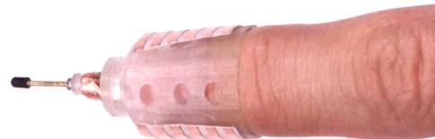
**Figure 13. A Capacitive touch sensor senses 1D gestures on each side of the NanoStylus.**
