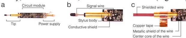
**Figure 5. a) Circuit of the active stylus removed from its body. b) Zoomed view of the tip. c) For the NanoStylus, shielded wire is used to separate the tip from the board; Copper tape forms the connection between the circuitry and human body.**
