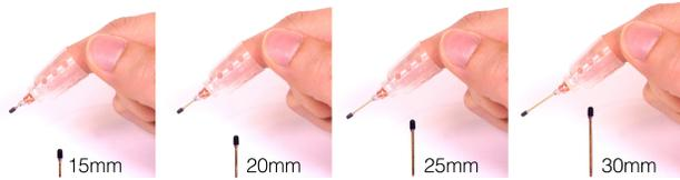
**Figure 7. The four nib lengths tested in the study.**
