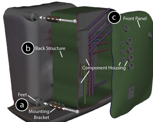
**Figure 11:** Exploded view of a RetroFab attached enclosure. The mounting bracket (a) is bolted to the mounting feet, which are glued to the legacy device. The back structure (b) holds the motors and sensors which interact with the new retrofit interface on the the front panel (c).
