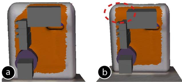
**Figure 3: (a) The orange region depicts the enclosure region that RetroFab derives based on the specified components. (b) The user manually extends the region to have additional space for the new shortcut button.**
