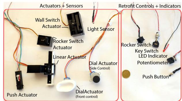
**Figure 8:** The RetroFab Toolkit; Left) actuators and sensors; the white material of the dial and linear actuator is the parametric component of the design which conforms to the scanned control. Right) controls and indicators.
