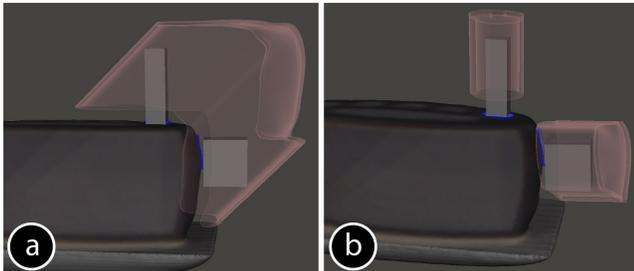
**Figure 13:** Depending on the surface region covered by the enclosure structure, users can decide to (a) combine actuators in a single enclosure, or (b) group some of them in a separate enclosure structure.
