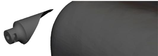
**Figure 14:** The mounting feet fit the curvature of the legacy object by using a Boolean difference operation with the scanned model.
