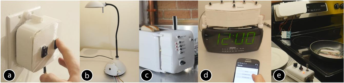
**Figure 15: Example retrofit interfaces created using RetroFab: (a) two wall switches, (b) a desk lamp, (c) a toaster, (d) an alarm clock with companion Android application, (e) an oven with remote enclosure.**
