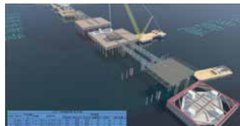
图16 Autodesk Navisworks 模拟主梁吊装与滑移
