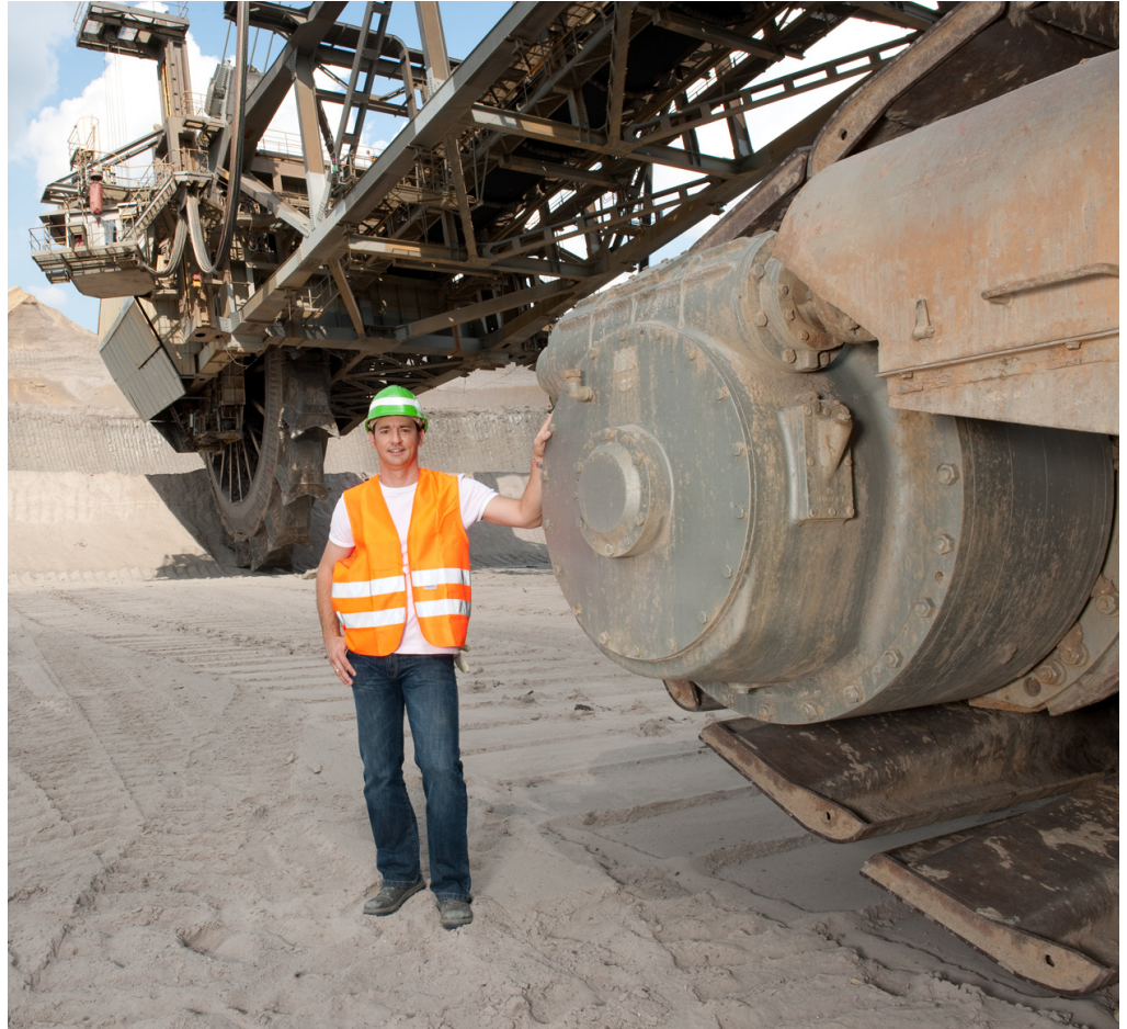
Peter Schnitzler, Engineer of Machine Technology, next to the crawler track assembly drive train (Photo: Autodesk)
