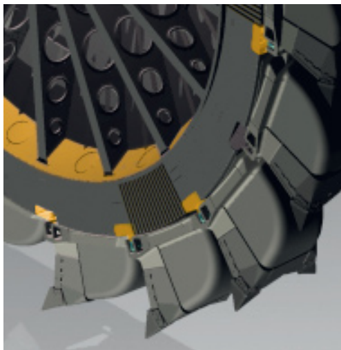
Detailed 3D representation of the bucket-wheel (Image: RWE Power)
