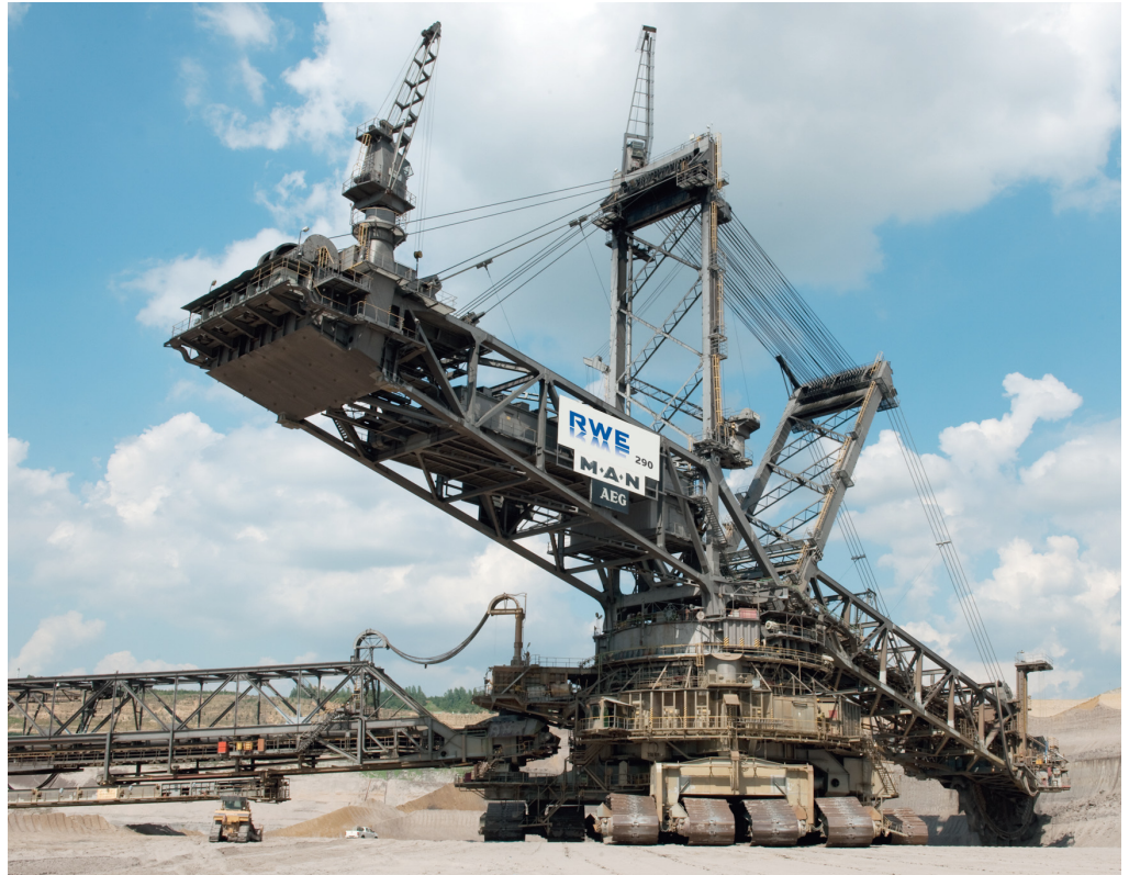
Bucket-wheel excavator 290 operating in the Tagebau Hambach strip mine; it can move up to 240,000 tons of coal or overburden a day (Photo: RWE Power)
