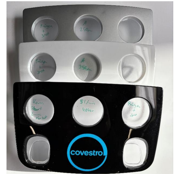
DE 250 \mu m partial compression molding + spot cooling
