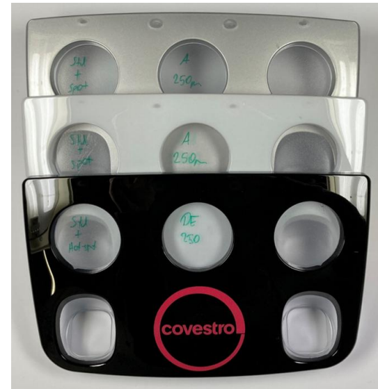
DE 250 \mu m standard molding + spot cooling
