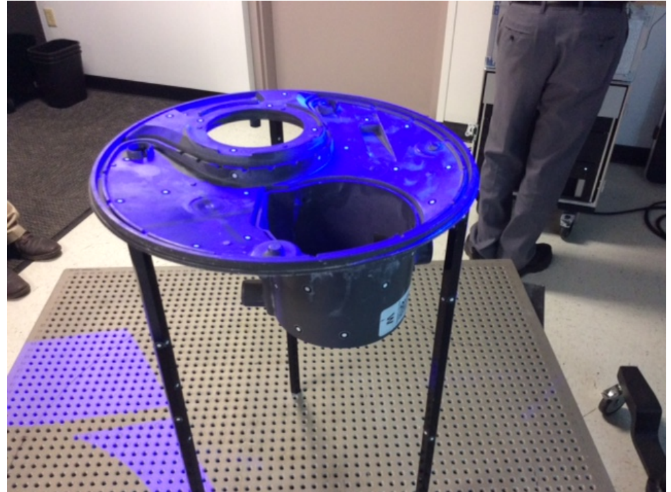
Blue Light 3D Scanning Simple Fixture. Part in free state
