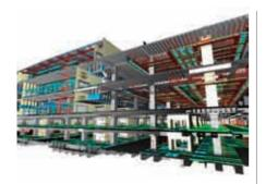
InteliBuild are BIM + 3D Specialists. Experienced professional engineers and knowledgable 3D CAD technicians collaborate to produce precise digital models for construction projects. The multi-disciplinary BIM models are used to identify design clashes and co-ordination issues. When combined with building programmes to create 4D models they can demonstrate site logistics and assist with construction planning.
