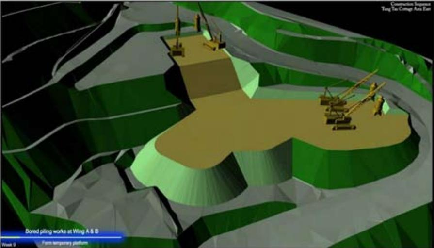
A detailed 4D virtual construction simulation was created to plan the construction sequence more thoroughly. Not only for the main building, a 4D virtual construction simulation was also created for the site formation and foundation system to ensure that the workflow is accurately planned.
