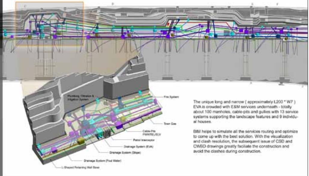
Using the BIM model, the main project team and the sub-contractors arranged the building services in much the same way as under the EVA: creating and refining a design with the services fitting into a small space, with access for maintenance, but without detectable clashes.
