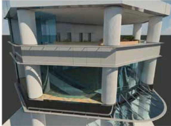
The BIM model for a Swire Properties development shows all project members the 3D appearance that would otherwise be only a mental image in the minds of one or two engineers. The model has helped to finalise the design, avoid clashes, and ensure smooth progress with construction in a small space accessed from a narrow, busy road.
