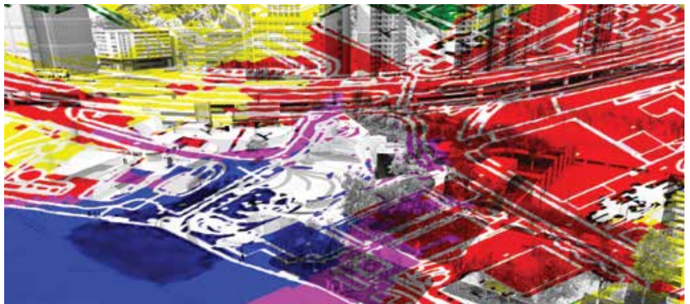
Noise mapping output for noise level distribution at noise sensitive receivers BIM is used as a tool to select the types of music acceptable for this cultural square Image courtesy of Architectural Services Department, HKSAR Government
