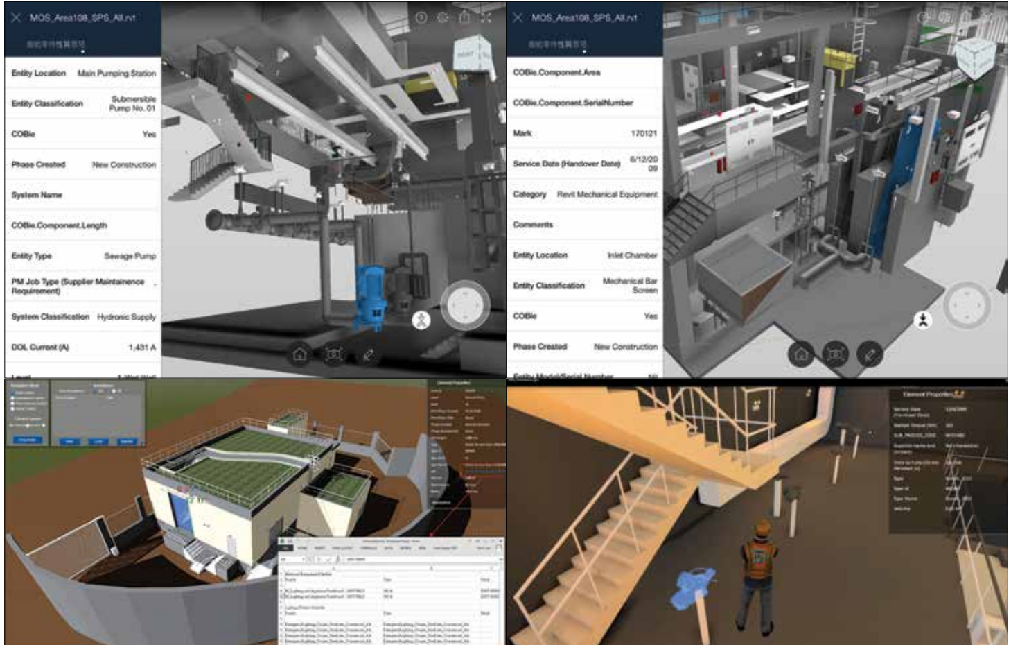
The digital asset information embedded in each model element Image courtesy of Drainage Services Department, HKSAR Government
