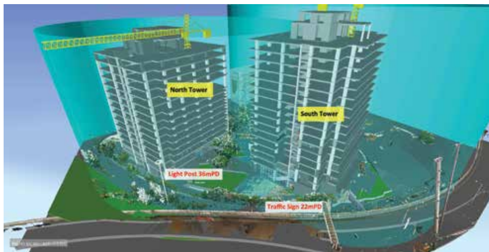
Tower crane working radius simulation based on integration of site condition scanning model and project BIM model Image courtesy of Hip Hing Joint Venture
