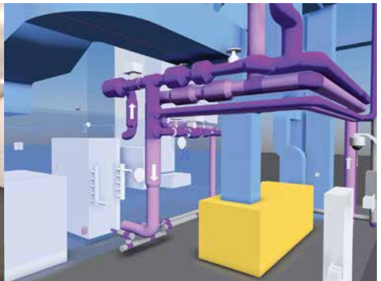
The BIM model of the AHU room providing HVAC services to the Lecture Theatre Image courtesy of Electrical and Mechanical Services Department, HKSAR Government
