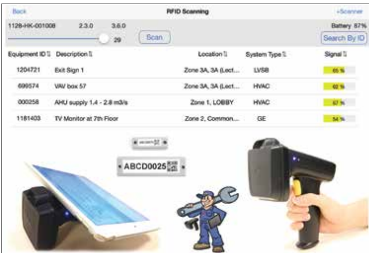
The screen capture showing the results of RFID scanning at mobile terminal for further enquiry of asset information Image courtesy of Electrical and Mechanical Services Department, HKSAR Government
