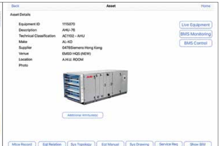
The screen capture showing typical asset details and features at mobile terminal Image courtesy of Electrical and Mechanical Services Department, HKSAR Government
