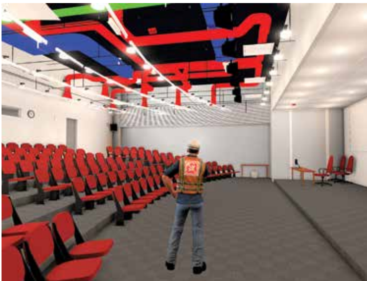
The BIM model of the Lecture Theatre of EMSD Headquarters Image courtesy of Electrical and Mechanical Services Department, HKSAR Government
