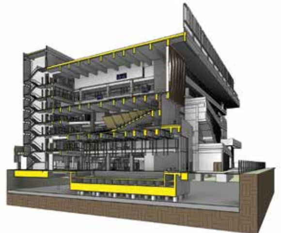
Malvern College. 3D section of the model with highlighted structure Image courtesy of P&T Architects & Engineers Limited
